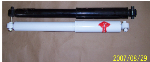
Note the extended lengths of the Gabriel “Classic” 82151(top) and the KYB Gas-adjust KG5197.
