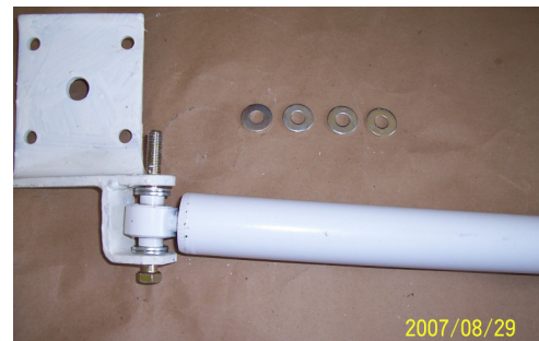
Bushings created from 4 3/8-inch washers.
